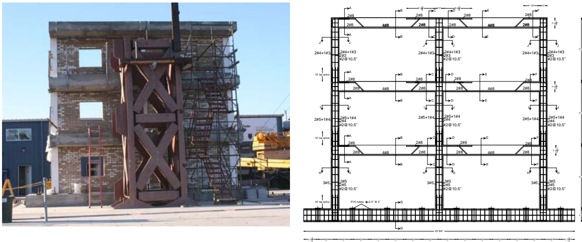
Figure 1 – 2/3-Scale Frame Tested on Shake Table
