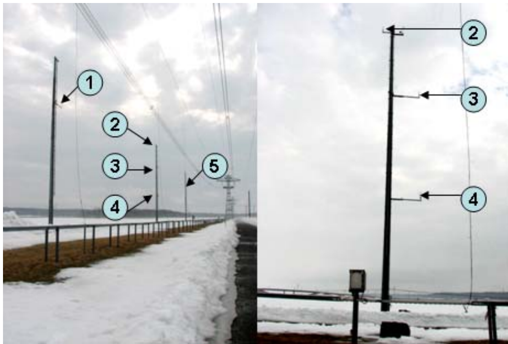
FIGURE 2 - SET-UP OF FIVE SONIC ANEMOMETERS FOR WIND MEASURE ON THE EXPERIMENTAL LINE OF IREQ
